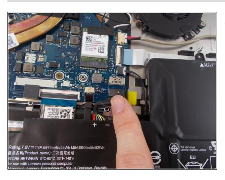
Remove the connector between the battery and the motherboard by gently pulling the black plasticcoated part of the wires.
