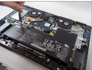
Remove the four 2 mm screws from the battery using a Phillips #0 screwdriver.
