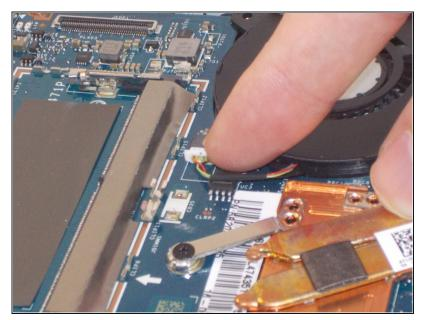
Unplug the wire connecting the fan to the motherboard by gently pulling the white head from the port.
