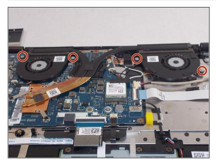
Remove the four 1.5 mm screws from the fans with a Phillips #00 screwdriver.
