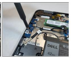
Remove the two 3 mm screws that secure the power switch board on the computer.
