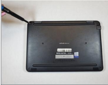
• Use a Phillips #0 screwdriver to remove the seven 7 mm screws securing the back case.
