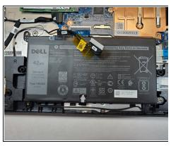
• Use a Phillips #0 screwdriver to remove the three 3 mm screws from the battery.
