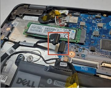
Disconnect the power switch cable from the motherboard.
