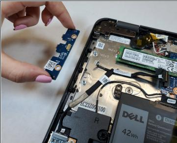
• Lift the power switchboard away from the computer.
