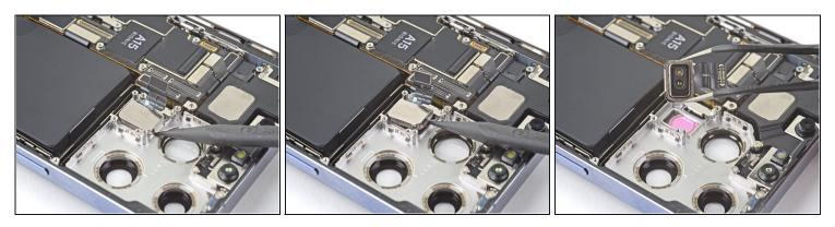
• Use the pointed tip of a spudger to lift the lidar sensor up out from the chassis and remove it.
