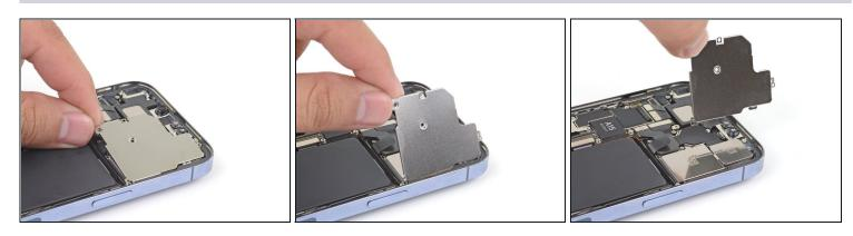
Lift the camera cover from the edge closest to the logic board, and remove it.
