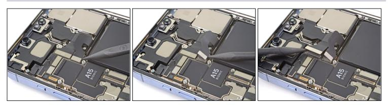
• Pry up with the pointed end of a spudger to disconnect the two camera cables from the logic board.
