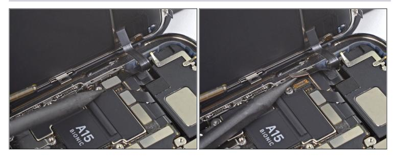
Use the pointed end of a spudger to disconnect the front sensor assembly cable connector.
