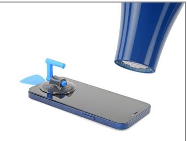
• Use a hair dryer to heat the right edge of the iPhone (the edge with the power button) for 90 seconds or until the screen is slightly too hot to touch.
