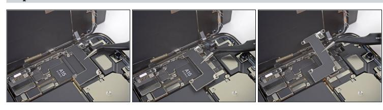
• Remove the front sensor connector cover.
