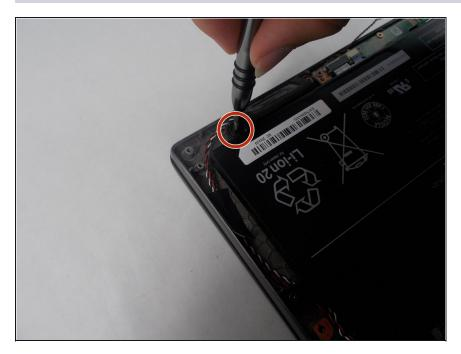
Remove the single 2 mm screw from the corner of the laptop using a Phillips #0 screwdriver.
