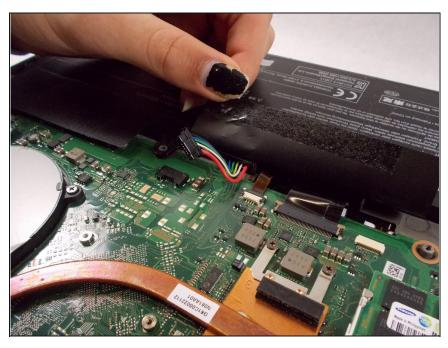
Pull the wired cable up towards the top of the laptop to disconnect it from its socket on the motherboard.
