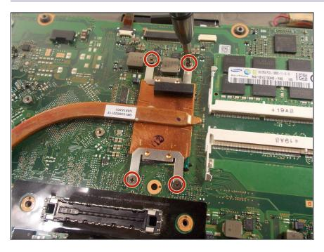
Remove the four 3 mm screws from the heat sink using a Phillips #0 screwdriver.
