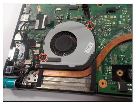
• Remove the two 4 mm screws from the fan using a Phillips #0 screwdriver.
