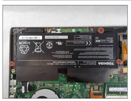
Remove the three 3 mm screws from the battery using a Phillips #0 screwdriver.
