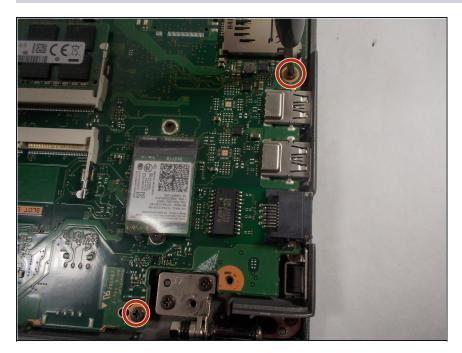
Remove the two 5 mm screws using a Phillips #0 screwdriver.
