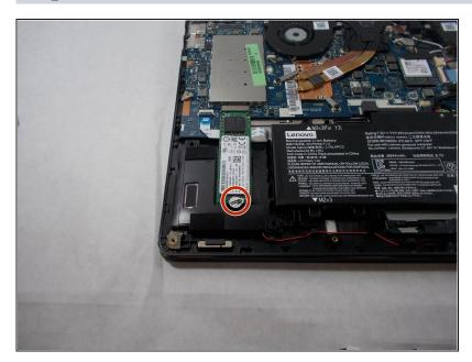
Remove the sticker from the SSD to gain access to the screw underneath.
