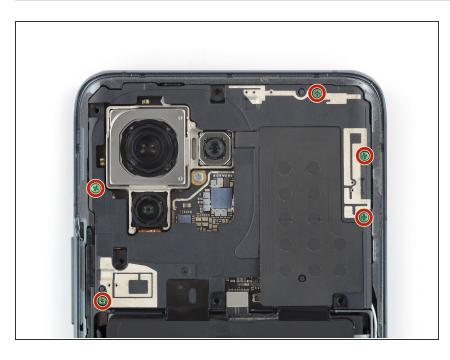
Use a Phillips screwdriver to remove the five 3.9 mm-long screws securing the motherboard cover.
