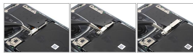
• Use a pair of tweezers to remove the connector bracket by pulling it in the direction of the battery.
