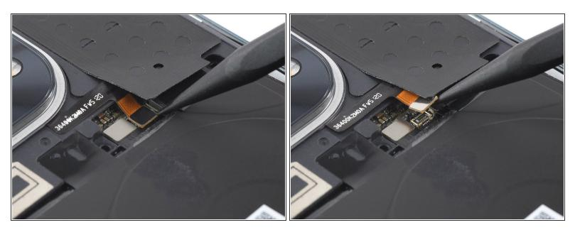
Use the pointed end of a spudger to disconnect the flash assembly cable by prying the connector straight up from its socket.
