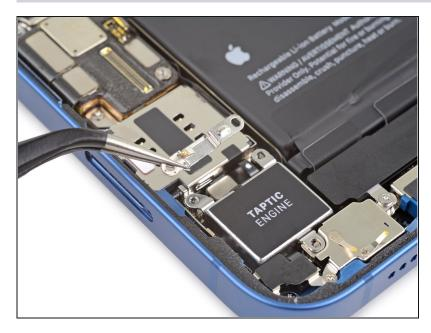
• Remove the Taptic Engine bracket from the top two screw hole tabs.
