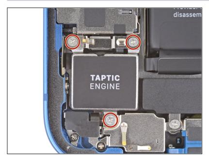
• Use a Phillips driver to remove the three 2.2 mm screws securing the Taptic Engine.
