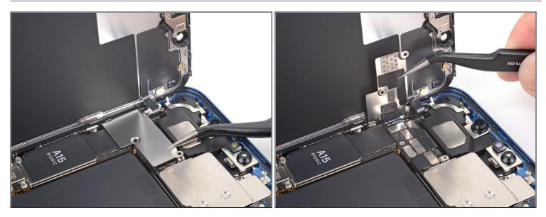
• Swing the cover up from the center of the phone until the small clip by the edge of the phone unhooks.
