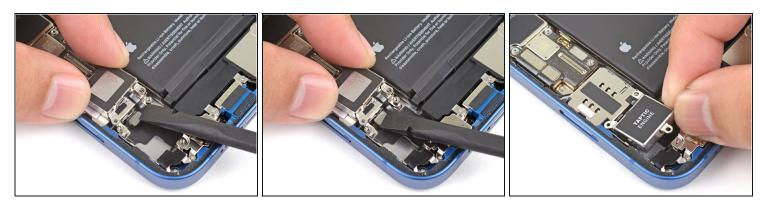
During reassembly, follow these steps to reconnect the Taptic Engine:
