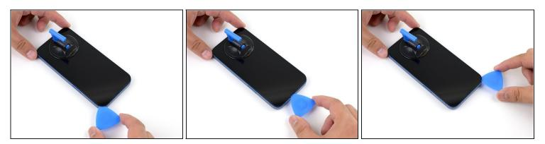
• Slide the opening pick around the top right corner of the iPhone to separate the top adhesive.
