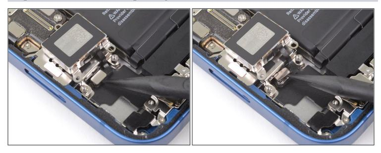
Use the point of a spudger to pry the Taptic Engine cable connector straight up and out of its socket on the logic board.
