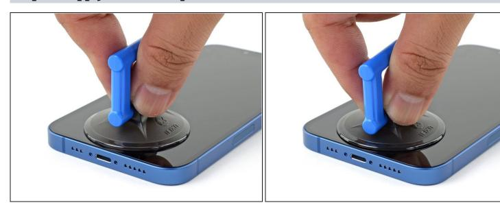
• If you're using a single suction handle, apply it to the bottom edge of the phone, while avoiding the very edge of the glass.
