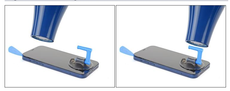
• Use a hair dryer to heat the left edge of the iPhone for 90 seconds or until the screen is slightly too hot to touch.
