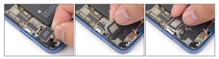
• Swing the Taptic Engine up from its lower edge so that it sits upside down on the SIM card reader.
