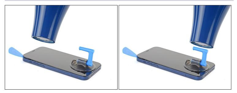
• Use a hair dryer to heat the left edge of the iPhone for 90 seconds or until the screen is slightly too hot to touch.
