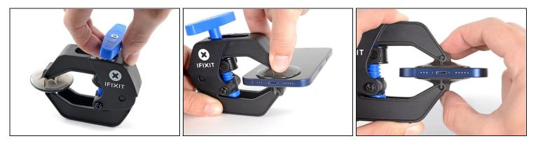
(i) The next three steps demonstrate <u>the Anti-Clamp</u>, a tool we designed to make the opening procedure easier. **If you aren't using the Anti-Clamp, skip down three steps** for an alternate method.
