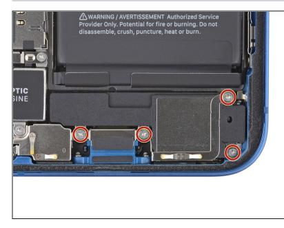
• Use a Phillips driver to remove the four 1.7 mm screws securing the loudspeaker.
