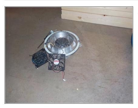
You can now remove the 4 P2 screws holding the fan down and then remove it from the light.
