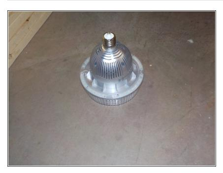
This is a 400W replacement HID to LED retrofit bulb from Keystone Lighting. It doesn't work anymore and has been replaced, so why not tear it down?
