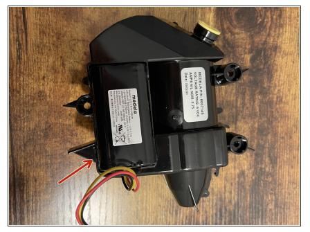
• The battery is attached to the black pump casing you just removed with adhesive.
