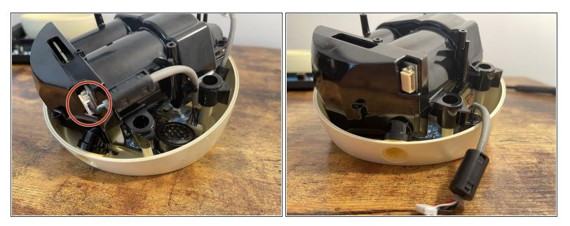
• Remove cable from port on the side of the black pump casing.
