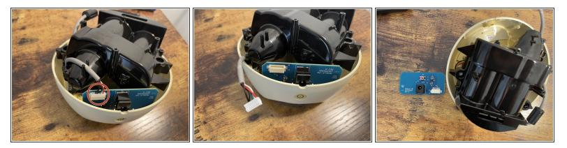
• Remove the cable from the blue board with the power button and charging port.
