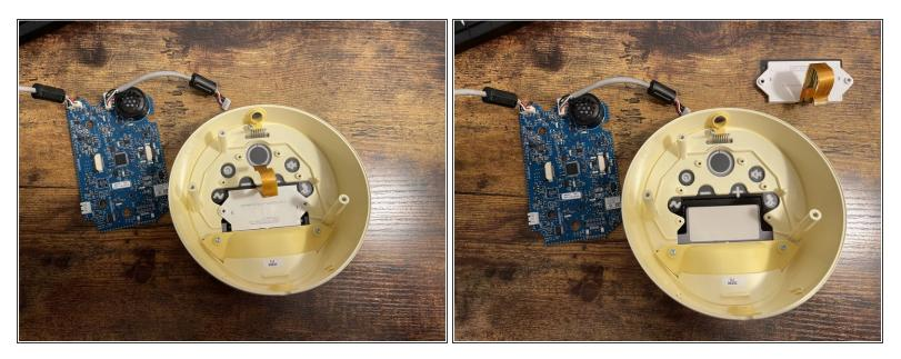
• Remove the main board and display panel.
