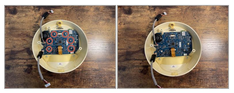
• Remove the 6 T10 screws from the main board.
