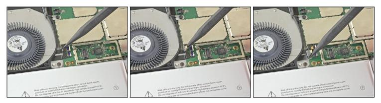
• Use the pointed end of your spudger to gently slide the fan and headphone jack cables out of their ZIF connectors.
