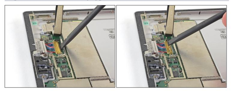
• Use the flat end of a spudger to flip up the retaining lock securing the charging assembly cable connector.
