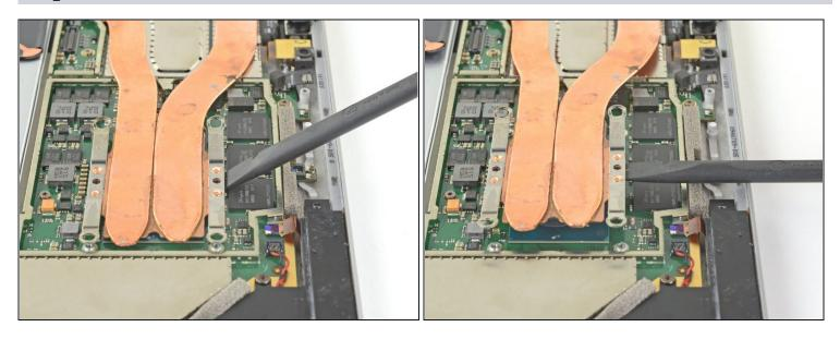
• Use the flat end of a spudger to gently pry the heat sink straight up and off of the CPU.
