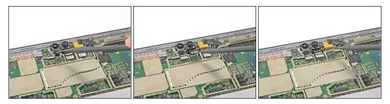
• Pry up with the pointed end of your spudger to disconnect all three camera cables from the motherboard.
