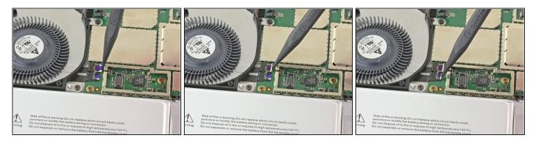
• Use the pointed end of your spudger to unlock the fan and headphone jack ZIF connectors.
