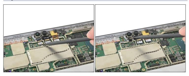
• Use the pointed end of your spudger to disconnect the IR camera from the motherboard.
