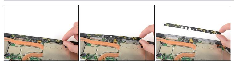
• Carefully remove the antenna support bracket.
