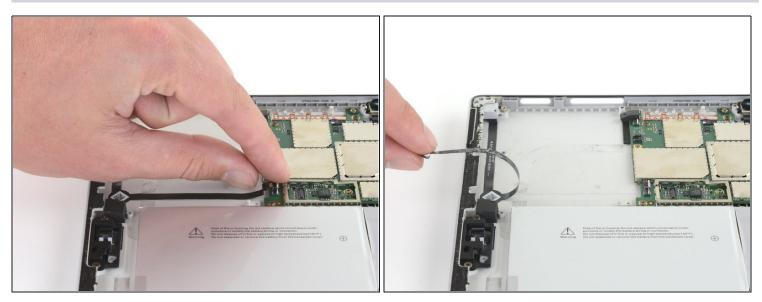
• Gently peel the headphone jack ribbon cable off of the case until you reach the corner of the cable.
