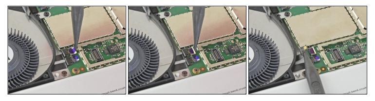
• Use the pointed end of a spudger to open the ZIF connector securing the fan to the motherboard.
