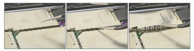
(i) Use this method to remove any EMI shields necessary during your repair:
