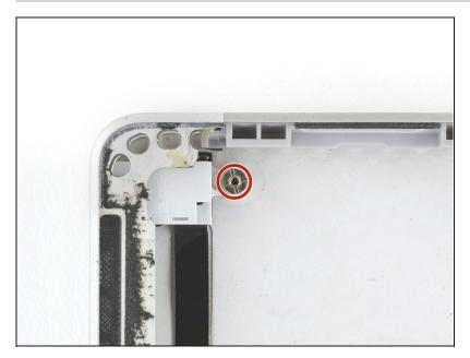
• Use a standoff screwdriver to remove the 4.3 mm screw securing the headphone jack to the case.
