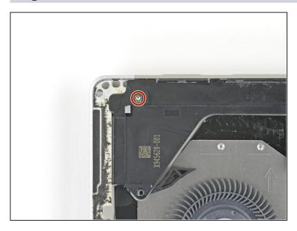
Use a T5 Torx screwdriver to remove the 3.3 mm screw securing the left speaker.
