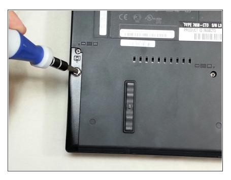
Using a #0 Phillips screwdriver, remove the 17 mm screw.
