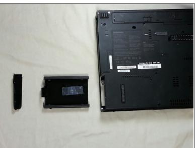
Pull gently on the black tab and the metal tray holding the hard drive will slide out.
