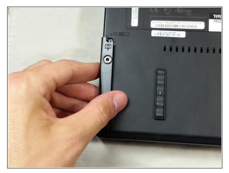
Carefully remove the plastic piece covering the hard drive by first pulling up then away from the computer.
