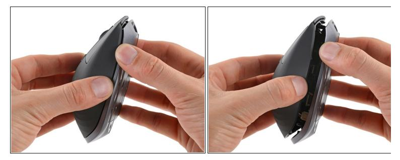
• Gently pry the upper shell and lower case apart to release the clips on the right side of the mouse.
