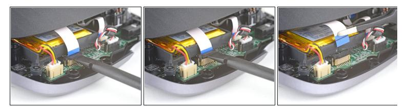
$\triangle$  Be careful not to strain the cable connecting the upper shell to the lower case.
