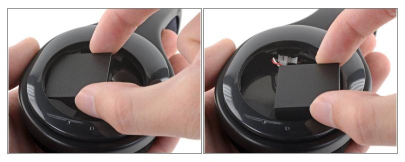
• Pull the battery to the right and away from the ear cup to remove it from the recess.
