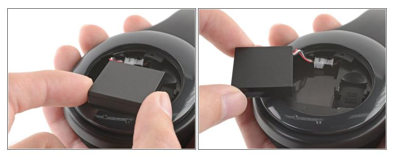
• Rotate the battery 90 degrees clockwise so that it rests on the left side of the ear cup.
