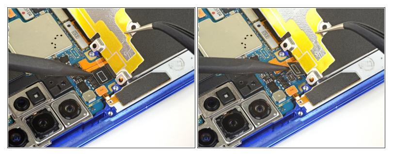
Use the pointed end of a spudger to disconnect the wireless charging coil connector from the motherboard.
