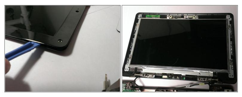
Slide the Plastic Opening Tool under the edge of the screen bezel to release the front panel of the screen.
