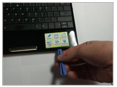
Using the plastic opening tool, carefully pry the top panel from the base.
