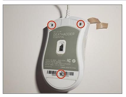
Close up the mouse, and replace the three 9 mm using a Phillips #1 screwdriver.
