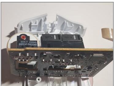
• This is the component that we will be replacing and its 3 contact points.
