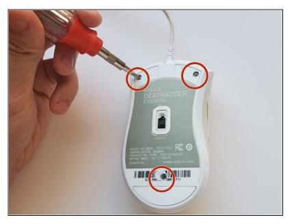
Use a Phillips #1 screwdriver to remove the three 9 mm screws that are holding the mouse together.
