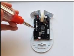
• Return the motherboard to its original position, and replace the two 11 mm screws and the single 4 mm screw using a Phillips #1 screwdriver.
