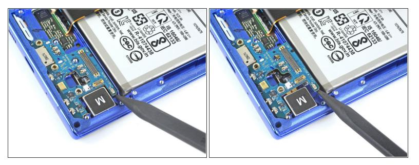
Use the pointed end of a spudger to pivot the daughterboard out of its recess.
