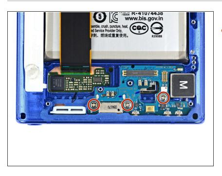
Use a Phillips screwdriver to remove the three 4 mm screws securing the charging assembly daughterboard.
