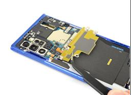
• Use a pair of tweezers to lift up and flip back the metal shield covering the battery connector.
