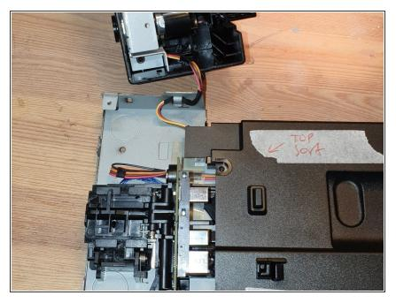
• Button assembly separated. The docking connectors are visible.
