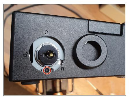
Pry off the bezel around the keylock. Remove the screw that connects the button assembly and the bottom assembly.
