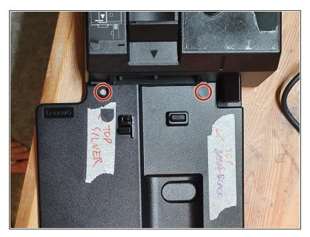
Use plastic picks or a metal spudger to pry off the top covers of the two screws on the top side.
