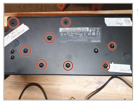
Remove the 8 bottom screws circled in red.
