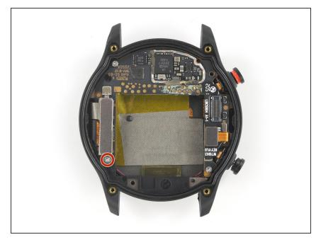
Remove the 2.7 mm-long Phillips screw securing the metal bracket at the bottom left corner of your watch.
