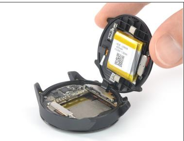
Carefully swing open the rear case assembly by folding the rear case to the side with the watch buttons.
