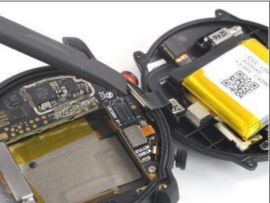
Use the flat end of a spudger to pry up and disconnect the rear case assembly flex connector from the motherboard.
