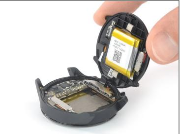
• Carefully swing open the rear case assembly by folding the rear case to the side with the watch buttons.
