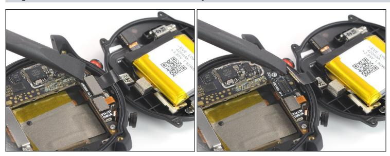
• Use the flat end of a spudger to pry up and disconnect the rear case assembly connector from the motherboard.
