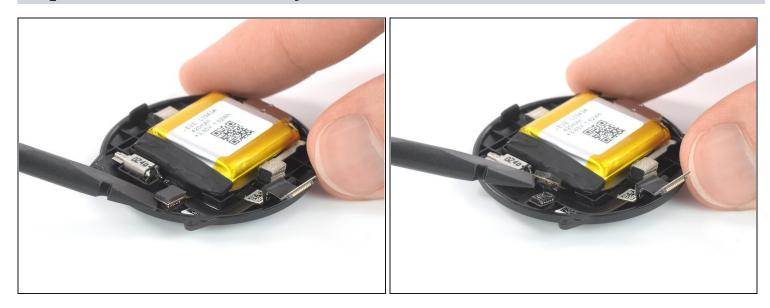
• Use the flat end of a spudger to pry up and disconnect the battery connector.
