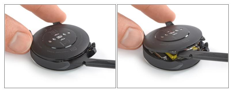
Insert your spudger into the gap and pry up the rear case assembly.
