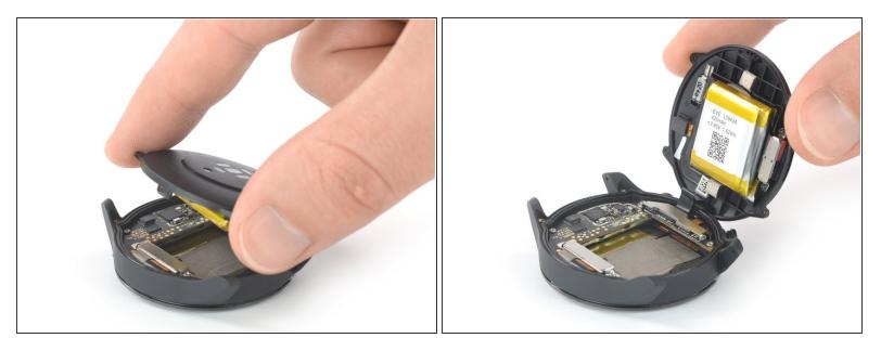
Carefully swing open the rear case assembly by folding the rear case to the side with the watch buttons.
