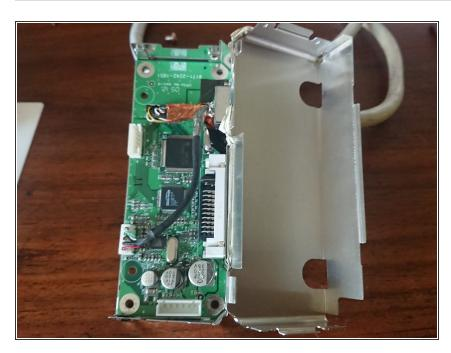
Unscrew the logic board and pull it out
