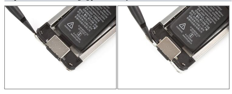
• Use the flat end of a spudger to shift the battery port assembly towards the bottom of the frame to free the metal clips holding it in place.
