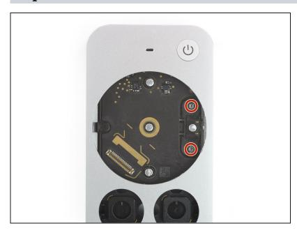
Use a T3 Torx screwdriver to remove the two 4.7 mm-long screws securing the Siri button on the right edge of the remote.
