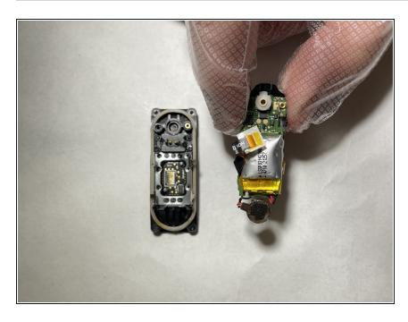
Remove the motherboard assembly from the device by gently lifting.
