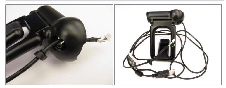
• Feed the end of the disconnected USB cable through the back cover.
