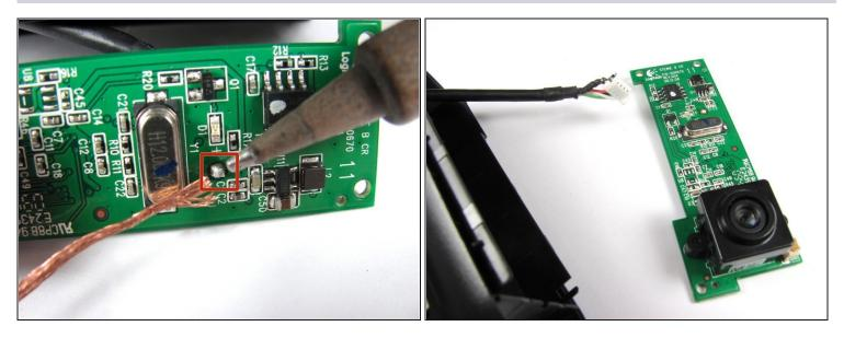
• Desolder the joint on the front of the motherboard to completely detach the USB cable.
