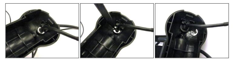
• Wedge the pointy end of the spudger between the sliver E-ring and USB attachment base to extract the E-ring and release the USB cable.
