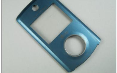
Separate the front faceplate from the device completely.
