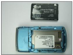
• Using your index finger lift and remove the battery from the phone.
