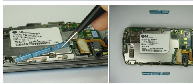
• Use tweezers to remove the volume control buttons on the opposite side of the phone.
