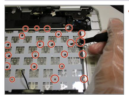
Remove all 52 screws from the keyboard panel using a Phillips #000 screwdriver.
