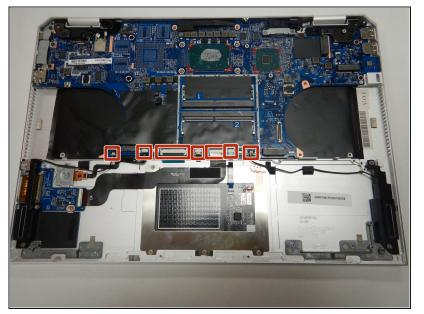
Unplug the seven ZIF connecters from the motherboard by flipping up the black switches with a spudger and pulling out the cables.
