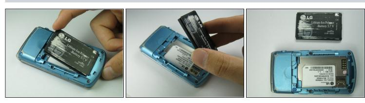
• Using your index finger lift and remove the battery from the phone.
