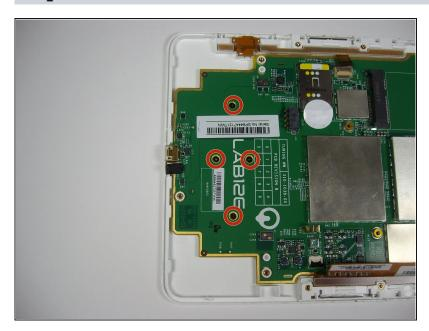
Use a Phillips #00 screwdriver to remove the four 4 mm screws from the motherboard located around the LAB126 logo.
