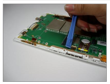
Locate the next brown connector three inches to the right of the previous connector and repeat Step 10 to remove the plastic ribbon.
