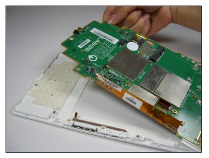
Grab the bottom corner of the motherboard and safely remove it from the Kindle.
