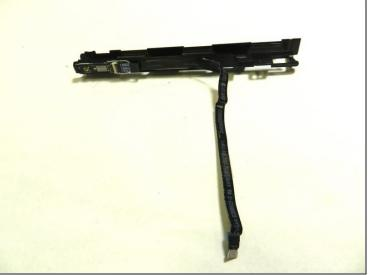
• Carefully lift out the digital pen holder with the attached power button ribbon cable.
