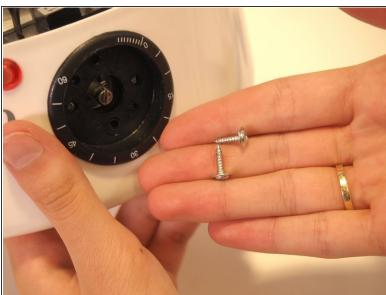
Using the JIS #1 screwdriver, remove the two 12 mm screws from the top and bottom of the timer socket.
