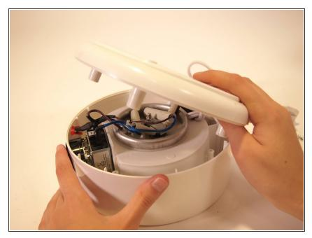
Once the four screws are removed, lift the bottom of the device off of the frame.
