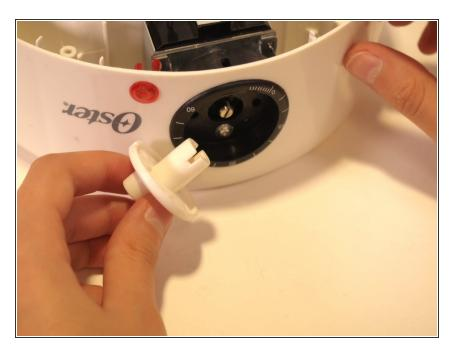
Pull the white dial the rest of the way out of the socket.
