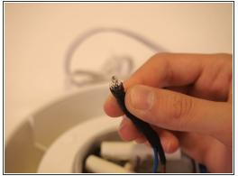
On the left-hand side of the device, carefully remove the indicator light from its place next to the timer by pulling on the heat protector covering the brown wire.
