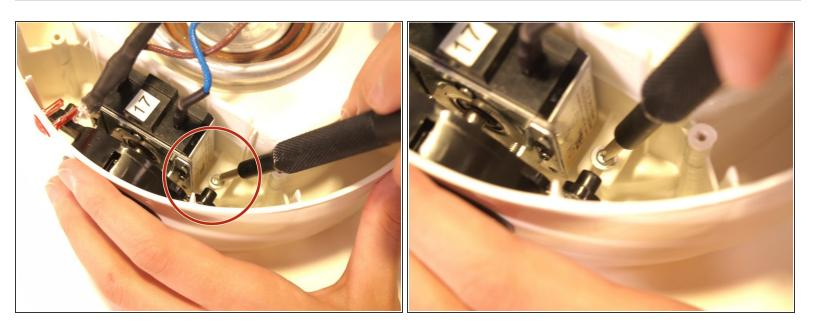
Using the JIS #1 screwdriver, remove the two 12 mm screws attached on each side of the timer.
