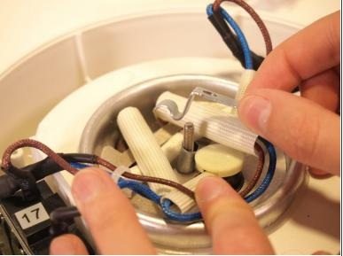
• Lift off the metal brace from the bolt in the center of the device.
