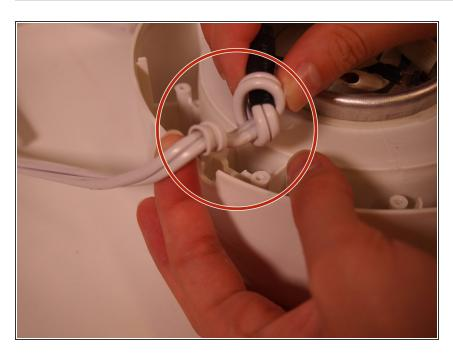
Lift the white power cord out of its socket.
