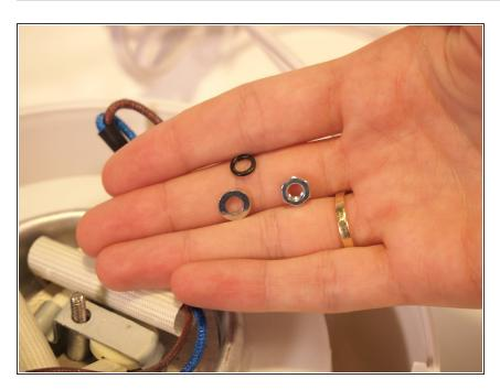
Remove the nut and the two washers from the center bolt.
