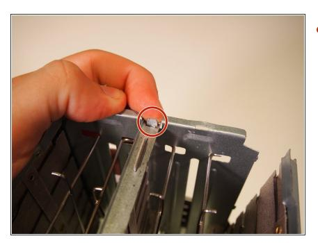
Unfold the two tabs on the top of the toaster that hold the central bar in place.
