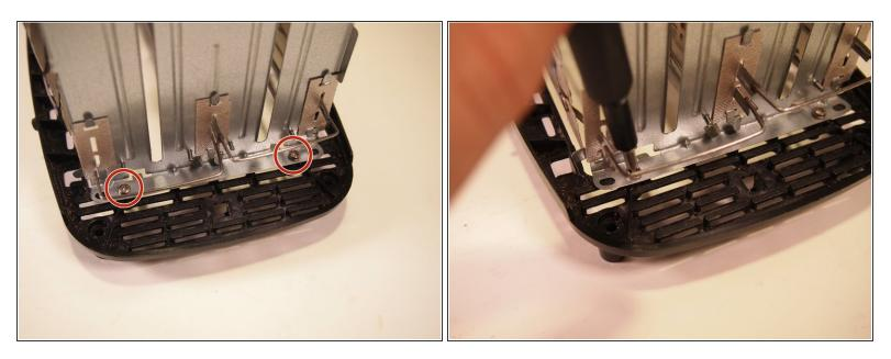
• Using the Phillips #1 screwdriver, remove the two 8.0 mm screws from the backside of the toaster.
