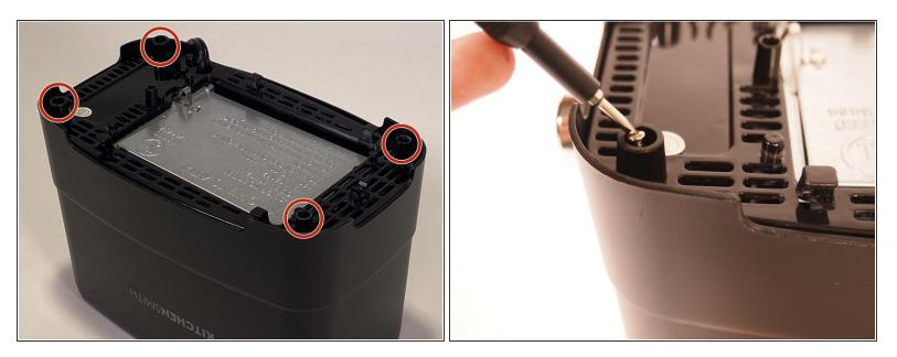
Using the Triangle #2 screwdriver, remove four 100.0 mm screws from the base of the toaster.
