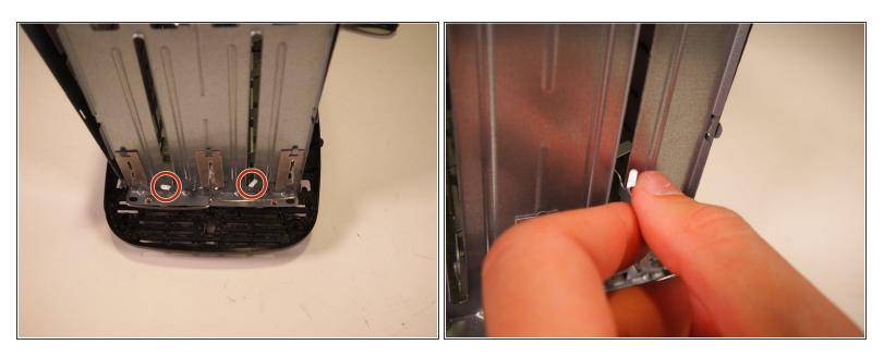
Unfold the two tabs on the back of the toaster.
