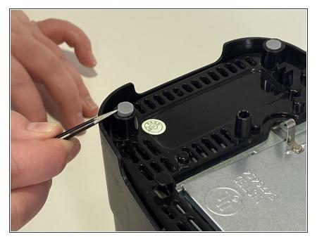
• Turn the toaster over. Remove the two rubber gaskets from the legs of the toaster using a pointed tool such as tweezers.
