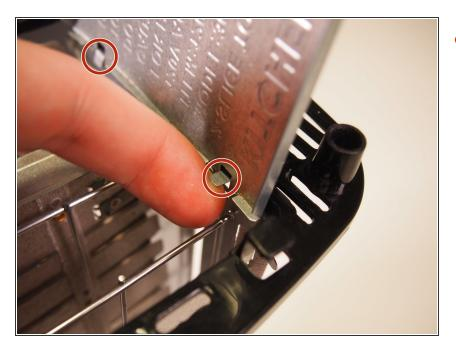
• Unfold the two tabs that hold the breadcrumb tray in place.
