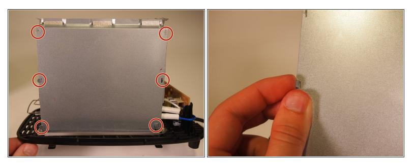
Unfold the twelve tabs that hold both sides of the toaster in place.
