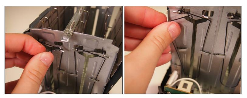
• Remove the spring part of the bread holding mechanism.
