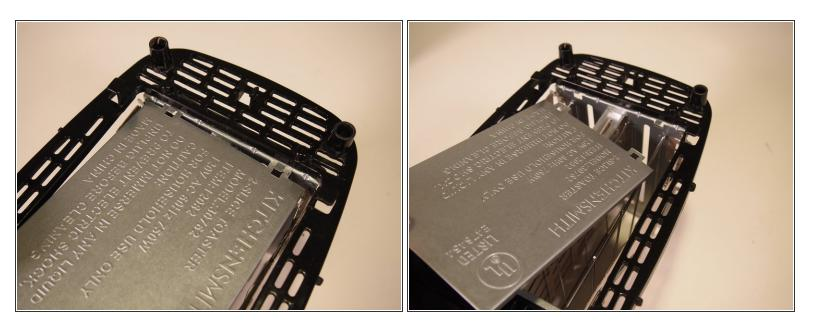
• Lay the tray back down to its resting position and then pull the tray up and away from the device.
