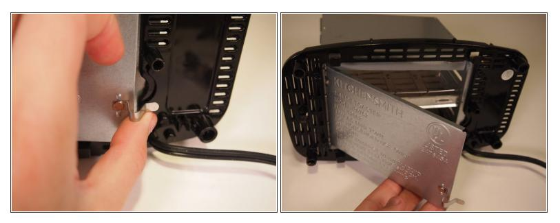
• Undo the latch to the breadcrumb tray and swing the tray open.
