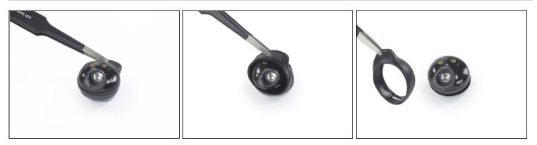
• Use your fingers or a pair blunt nose <u>tweezers</u> to remove the earbud's rubber wingtip by pulling it upwards while slipping it off the earbud.
