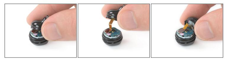
A Make sure that the flex cable is not under tension during the following step.
