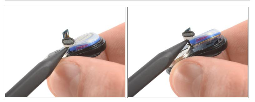
Use the pointed end of a spudger to slightly lift up the speaker driver obscuring the battery.
