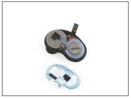
Use a spudger or your fingers to remove the plastic frame by pulling it upwards.
