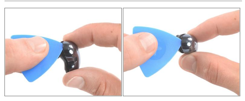
Keep the opening pick at a steep angle and slide it along the top to loosen the case.
