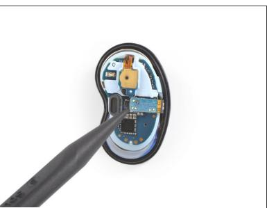
Use the pointed end of a spudger to lift up and disconnect the main connector.
