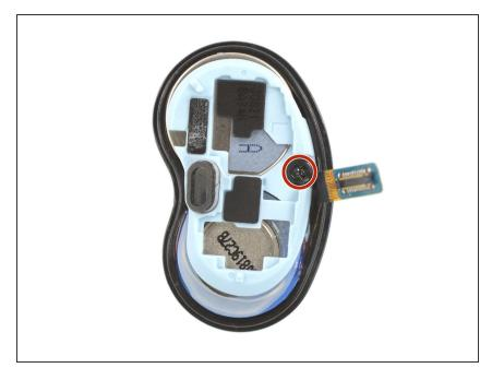
Use a Phillips screwdriver to remove the 3.4 mm-long screw which is securing the plastic frame.
