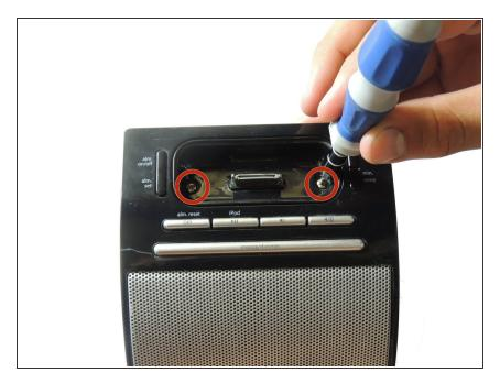
Remove the two 9mm screws from the top of the iHome with a Phillips #1 Screwdriver.
