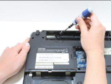
• Remove the three 3mm Phillips #1 screws inside the battery compartment.
