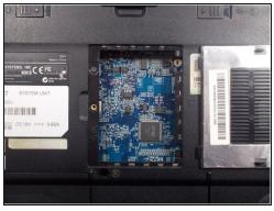
Use a plastic opening tool to open the motherboard access cover.
