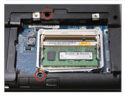
Unscrew the two 8mm Phillips #1 screws inside the RAM compartment.
