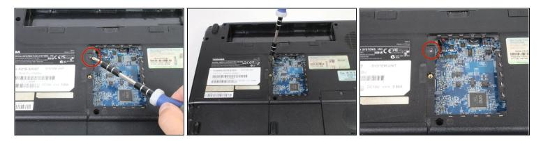
• Remove one 1.5mm Phillips #1 screw located near the top left edge of the opening.
