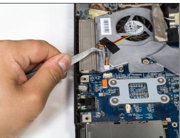
• Using tweezers, disconnect power cable by gently pulling white end straight away from its socket.
