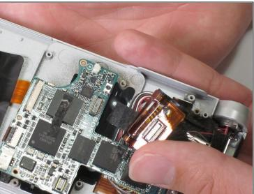
• Unplug the ribbon cable connected at the bottom of the memory module by prying it up with a spudger.
