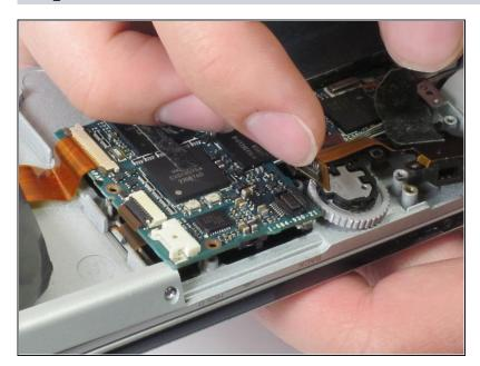
Unplug the audio module from the motherboard by disconnecting the wires by lifting the orange wire up.
