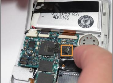
• Use <u>tweezers</u> to unplug the speaker wire from the motherboard by pulling the plug (not the wires) down towards the speaker.
