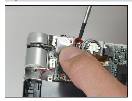
Unscrew the 2.5mm screw on the top portion of the audio module with a Phillips #00 screwdriver.
