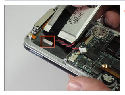
Gently peel back the adhesive to completely disconnect the battery pack from device.
