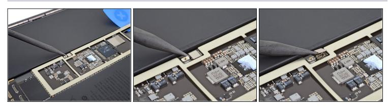
Use the pointed end of a spudger to disconnect the Smart Connector cable by lifting straight up on the press connector.
