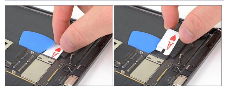
• Remove the battery blocker.
