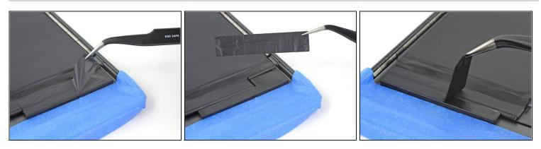
• Use a pair of <u>tweezers</u> to remove the two pieces of tape securing the battery to the lower buffer blocks.
