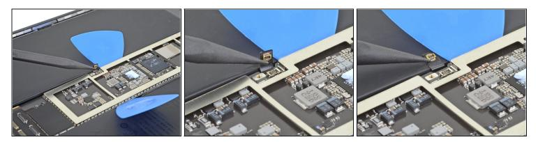
Use a spudger to move the Smart Connector cable behind the opening pick.
