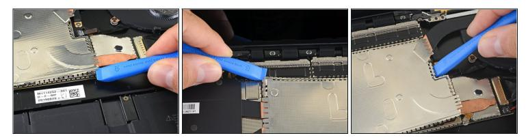
• Work your way around the perimeter of the shield, prying up intermittently, until you can remove it completely.
