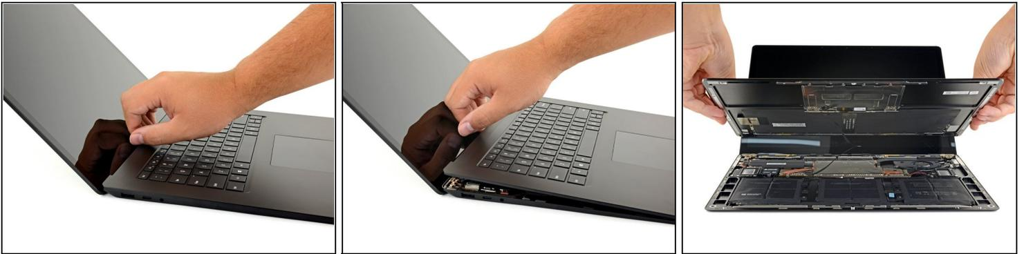
**i** The upper case is secured in place by magnets.
