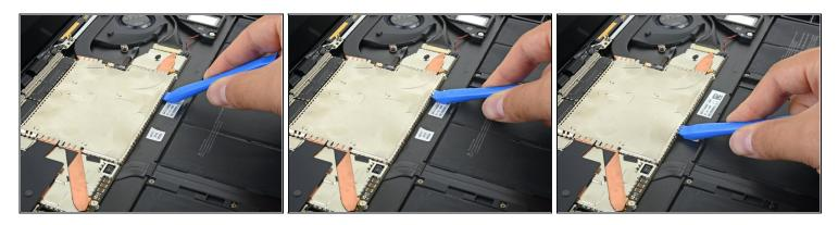
• Use an opening tool to pry up the front edge of the metal shield covering the heatsink.
