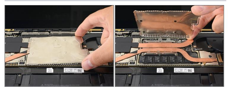
• Remove the heatsink shield.
