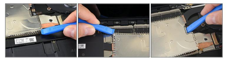
• Work your way around the perimeter of the shield, prying up intermittently, until you can remove it completely.
