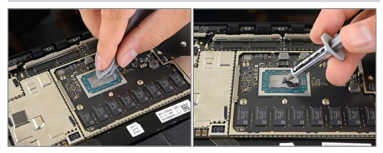
Before reinstalling the heatsink, follow this guide to clean the heatsink and CPU and reapply thermal paste.
