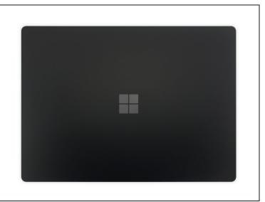
Turn on your laptop and allow the battery to discharge below 25% before starting your repairs, as a charged lithium-ion battery can be dangerous if accidentally punctured.
