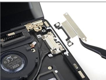
• Remove the Surface Connect port cover.
